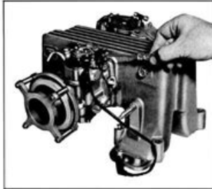
Fig. 10 Disconnecting Starting Cut-Off Switch
