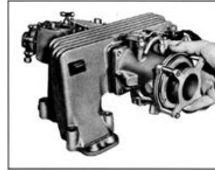
Fig. 11 Removing Air Meter
